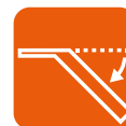
Break-back wrench with wider angle; longer time to stop after reaching target torque avoiding over-torque
